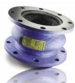
**Style 204 and 204HP Expansion Joint** Styles 204 and 204HP spool-type expansion joints can be constructed as single or multiple arch types. They connect pipe flanges in concentric or eccentric tapers, to join piping of unequal diameters.
