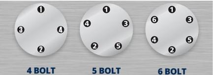
**NOTE:** Bolt torque is expected to lose roughly 5% to 10% of initial capacity after installation. Repeat torquing to the above corresponding torque range is recommended for customer confidence after a minimum of 24 hour time.
