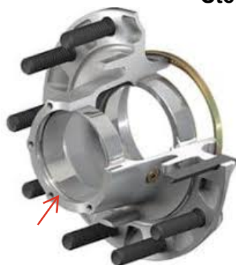
Short Snout Small gap between mount surface and bearing cup
